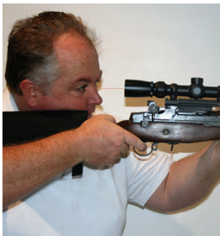
With the rifle cleared, the magazine removed and action locked open, Daniel O'Dea demonstrates cheekweld and the line of sight relationships with the Bistoli Adjustable Cheek Piece installed.
